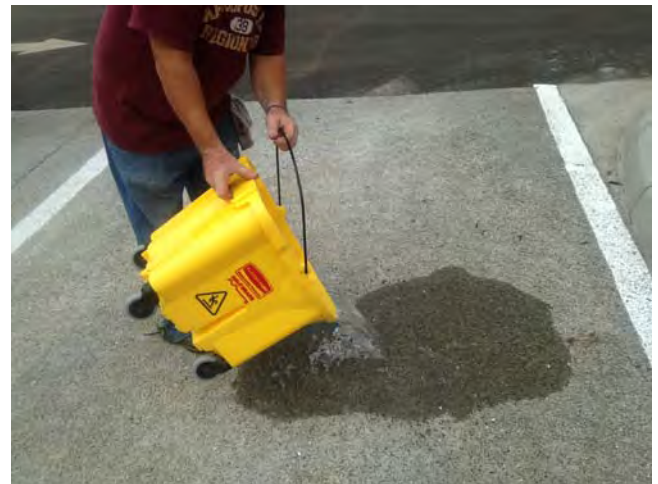
Testing Pervious Concrete Parking Space at Commercial Facility in North Port
