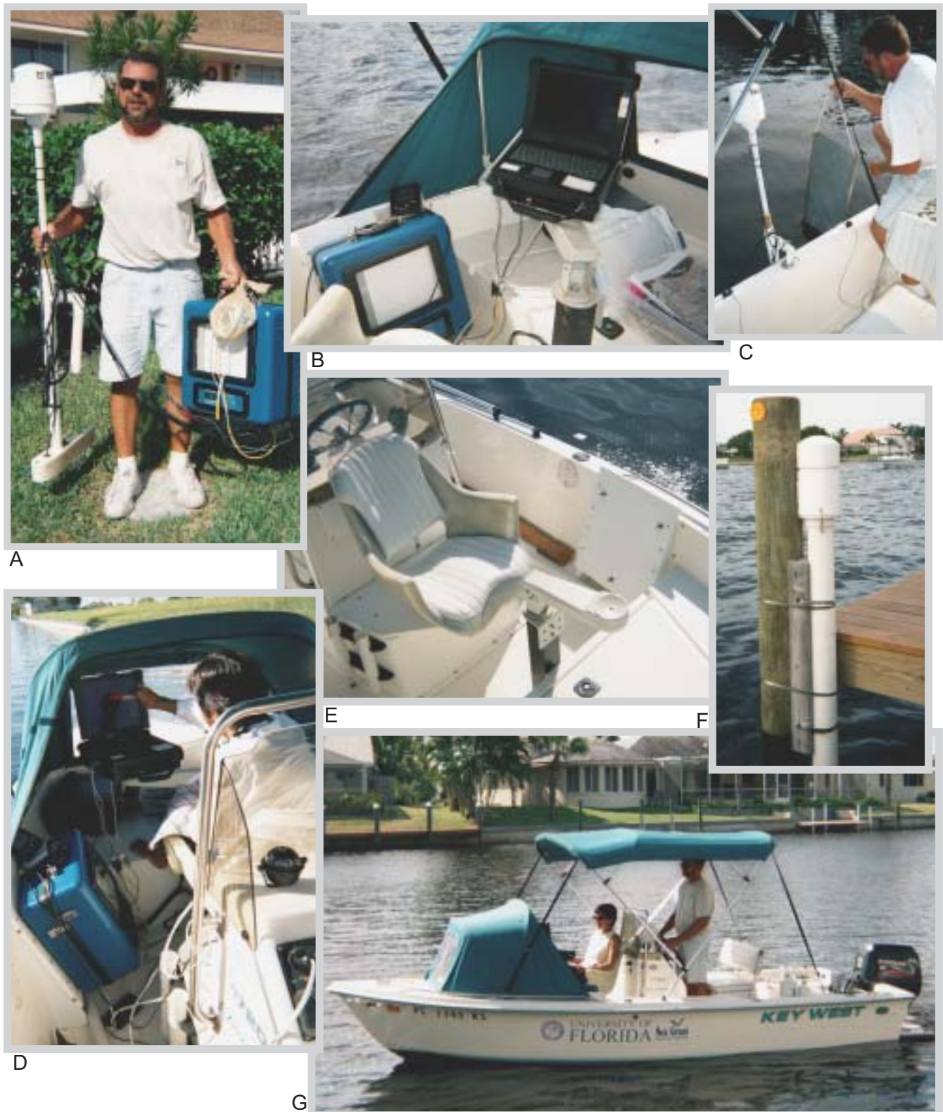
A. Bathy 500-MF Sounder, Transducer, and DGPS Antenna B. Data Collector's Work Station C. Bar Check D. Data Collector During Soundings E. Data Collector's Chair and Bathy Sounder Mount F. Infinities Portable Tide Gauge and Stilling Well G. Key West 17-foot Boat
