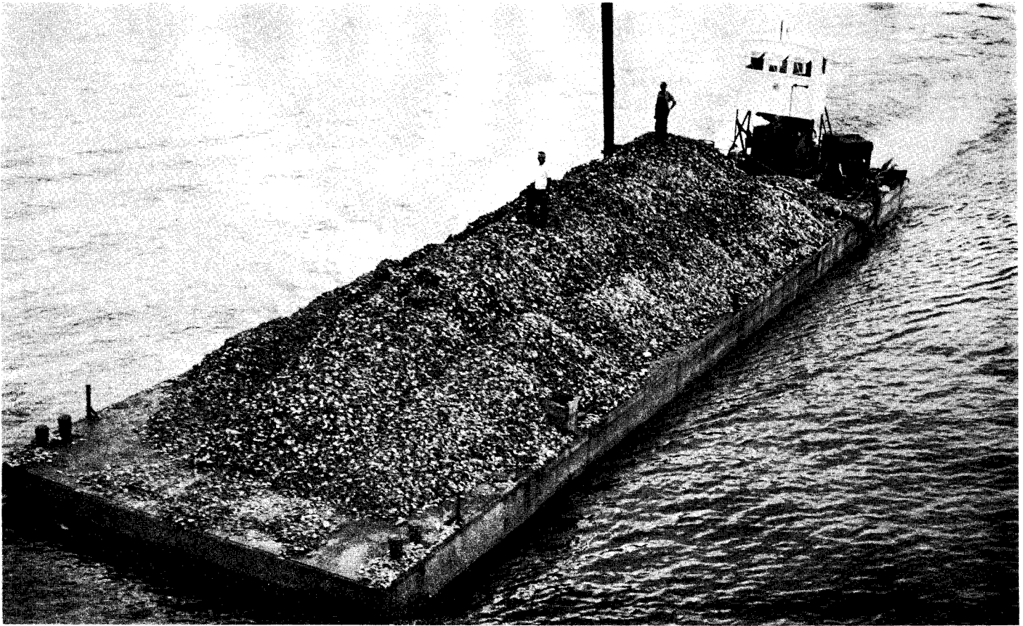
Figure 1. Self-propelled barge loaded with shucked shell under way to a planting site in Apalachicola Bay.
