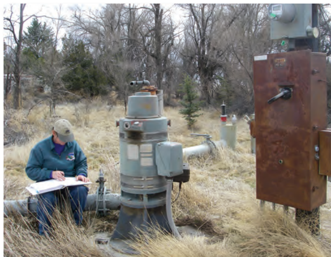
Water levels are recorded from an irrigation well in Laramie County, Wyoming.
