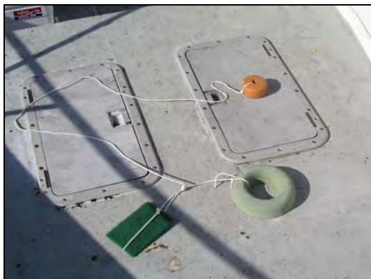
Fig 7. Recruitment collector including weight and surface buoy
