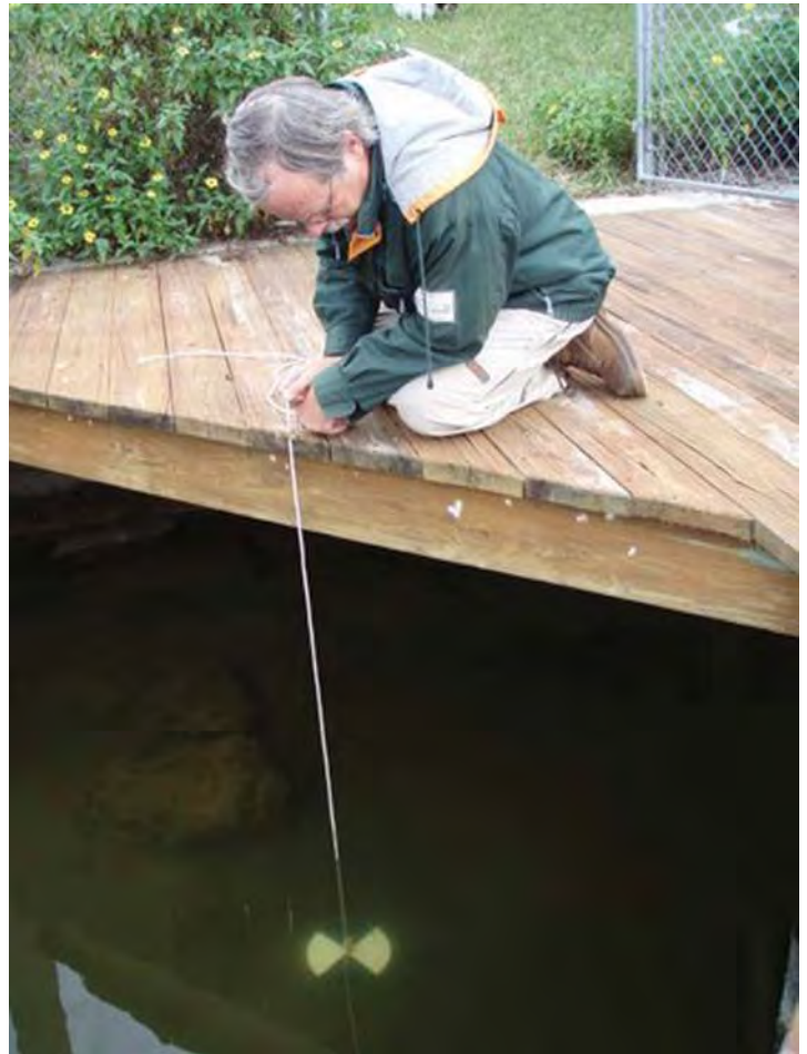
Carey Parks takes a Secchi depth reading. This circular disk has been used since 1865 to measure water transparency. It measures how deep a person can see into the water. Photo taken by Ruth Parks.
