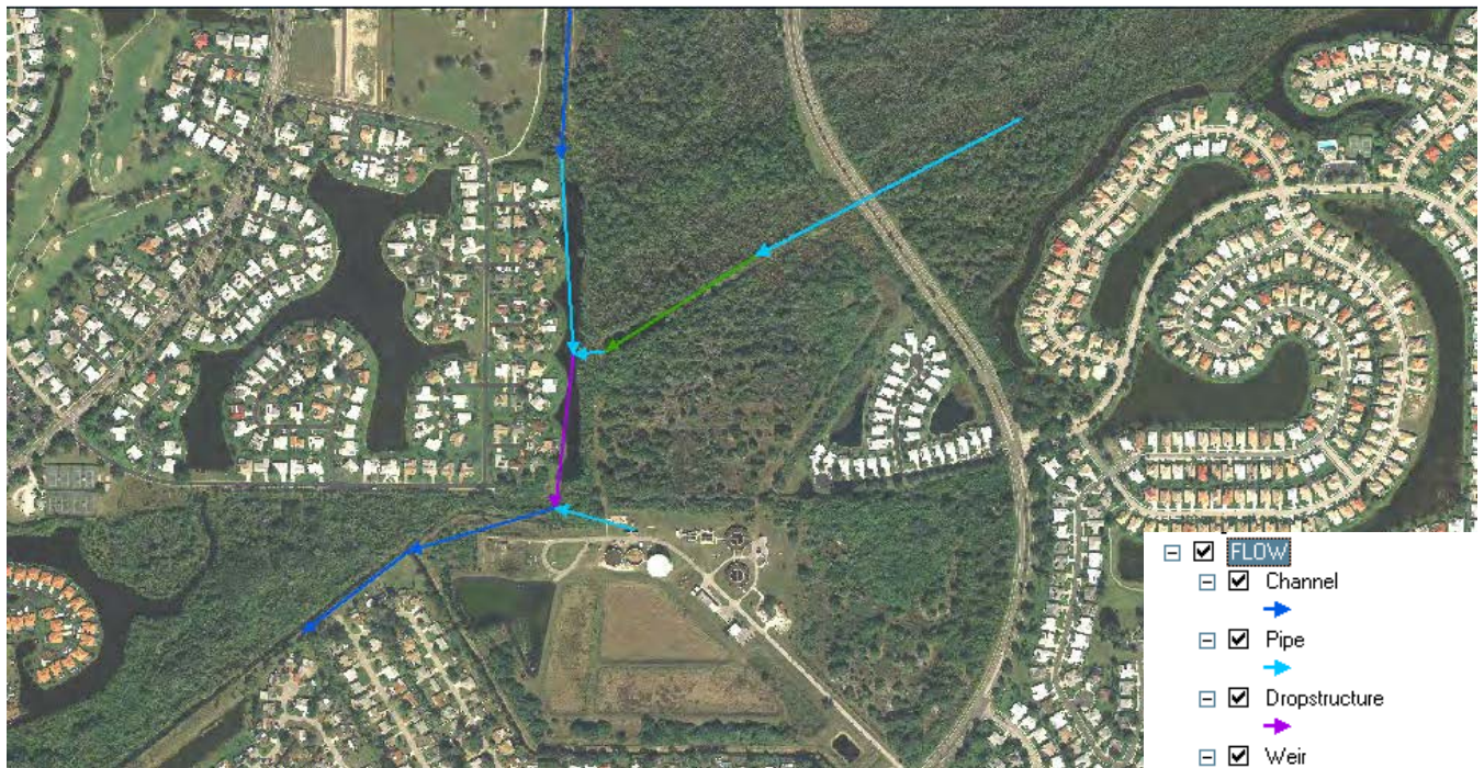
Figure 4-61 Existing Creek Rerouted Through Pipes, Stormwater Ponds, Drop Structures, and Ditches
