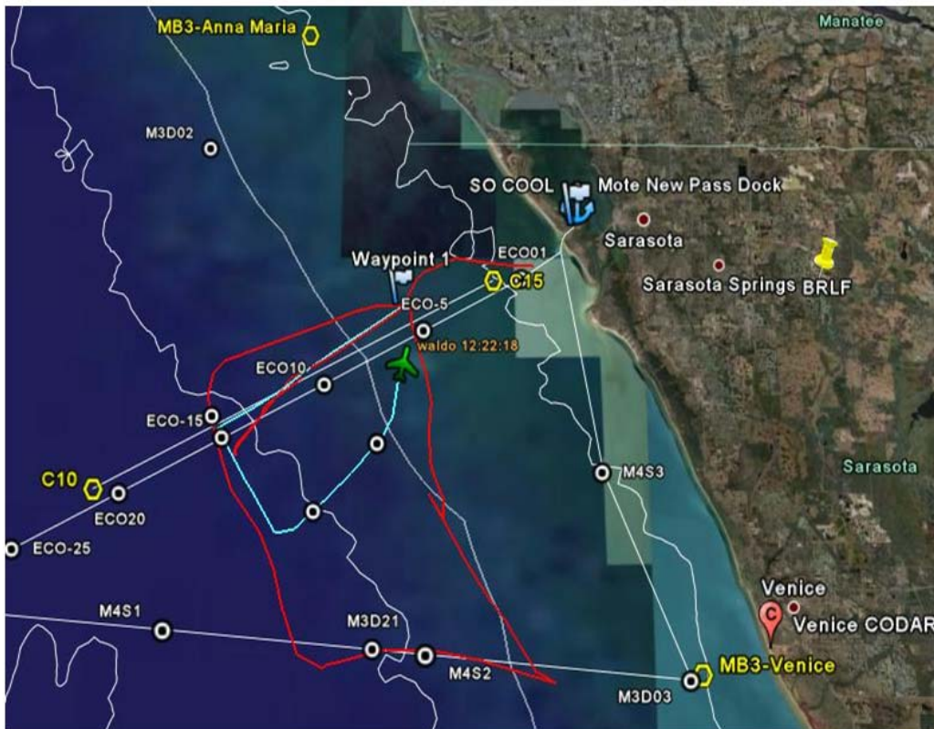
Figure 24 The tracks followed by the Slocum glider Waldo (SN045) during missions July 23 to August 4, 2008 (red line) and September 3 - 6, 2008 (light blue line). Yellow hexagons indicate locations where BreveBusters were deployed on buoys.
